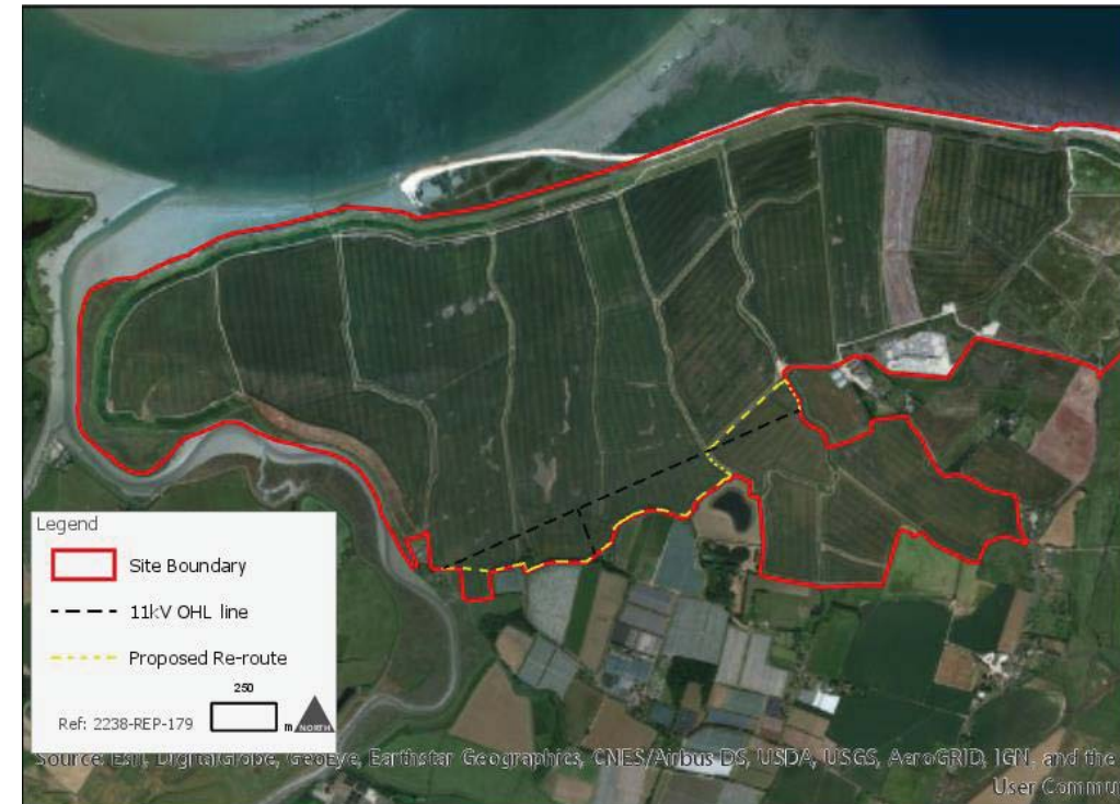
Figure 1: Existing OHL Route and Indicative Undergrounding Route
